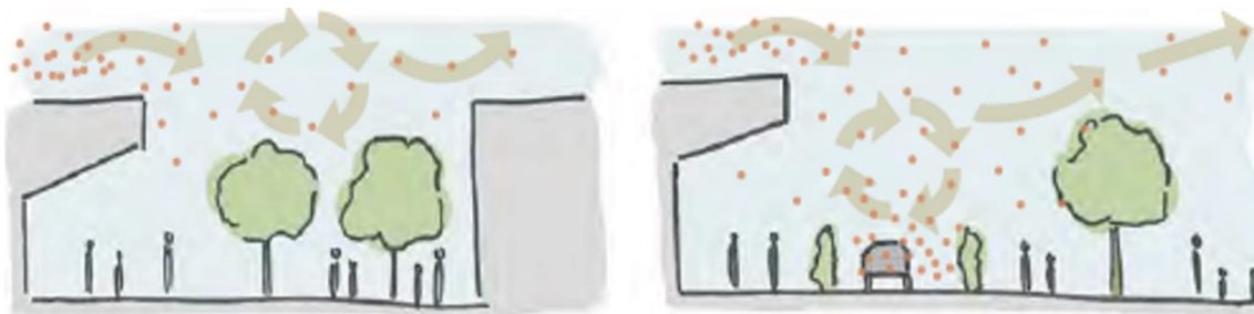
Figure 3.6: Street canyon where air above the buildings is more polluted than the air at street level
