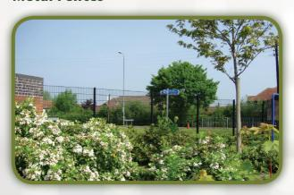
**Welded mesh** fencing creates a secure boundary. Using a smaller mesh will increase the security if required. Dark coloured fencing is less visible than a galvanised finish, softens the appearance of metal fencing and makes it easier to see through.
