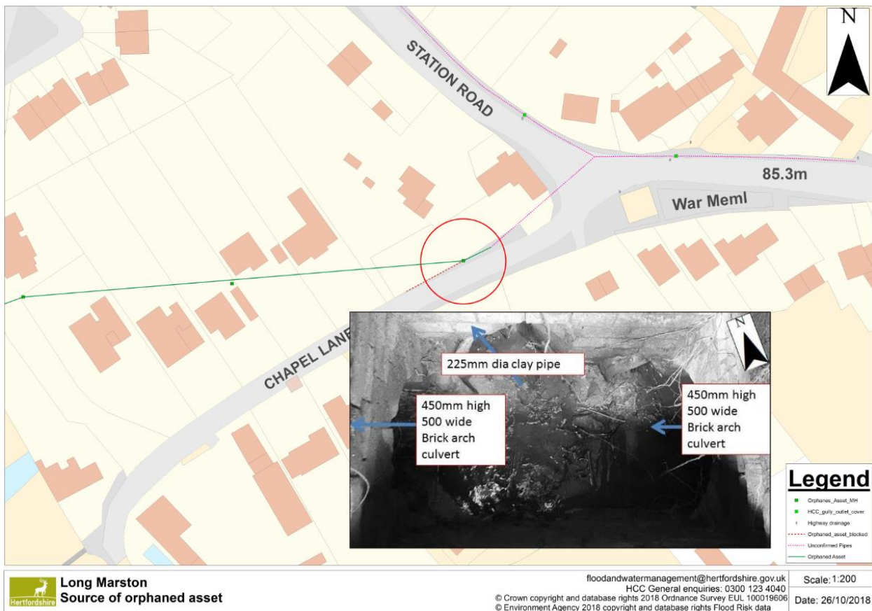
Figure 17 Silt and issues of structural integrity in culvert
