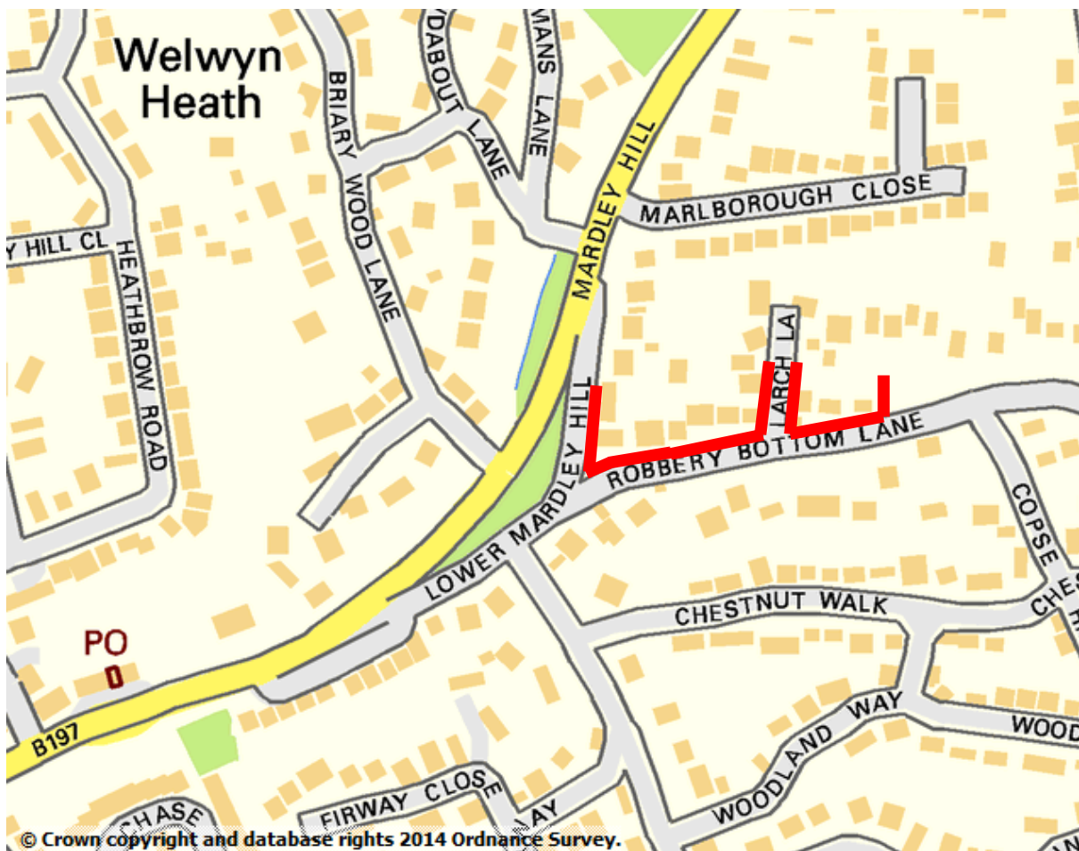
Figure 14 Recommended location of flood wall (background taken from OS OpenData on 02.09.2014)
