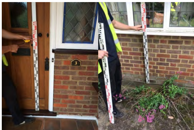
Surveying of property threshold levels for use in flood modelling
