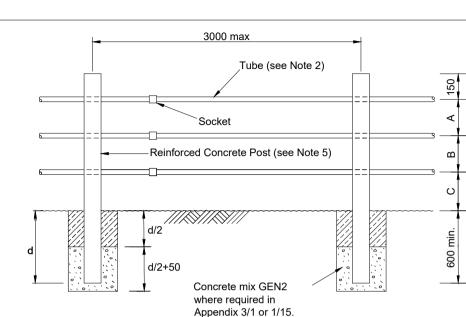
**DIMENSIONS** TYPE NO.OF POST REF TUBES SECTION C 3A 3 405 405 410nom 200x200 3B 3 375 375 250 200x200 2A 2 400 350 175x200 500 2B 2 500 200x200
