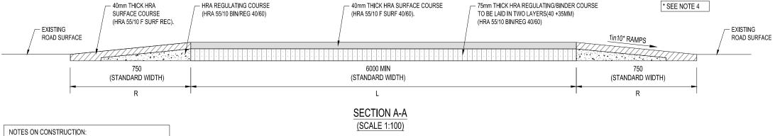
HUMP AND PLATEAU TO BE MACHINE LAID. PLATEAE PLATEAU TO BE CONSTRUCTED FIRST IN TWO LAYERS. PLATEAU TO BE LARGER THAN SPECIFIED SO THAT IT CAN BE SAW-CUT BACK ON ALL SIDES BEFORE CONSTRUCTION OF THE RAMPS, EXISTING MATERIAL TO BE REMOVED AS SHOWN TO CONTRACTORS LICENSED TIP OFF SITE.
