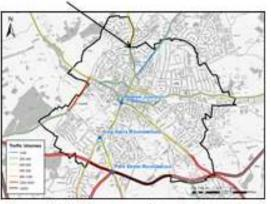
Figure 10: Traffic volumes in the St Albans urban area, AM Peak (08:00 - 09:00). Source: OS Data @Crown Copyright (and database right) (2016): Trafficmaster 2014-2015 AM Peak (0800-0900) data.
