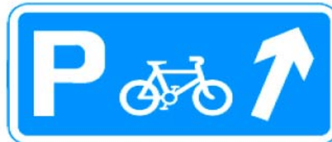
Figure 10 – TSRGD Diag. No. 2603 used to highlight the location of cycle parking
