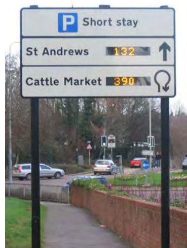
An example of a real time parking information sign
