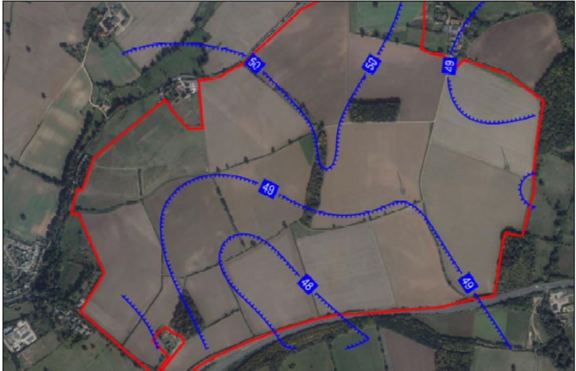
Figure 58: Groundwater Level Contours
